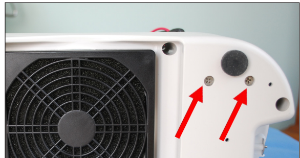
Figure 66 - Step 6 Unscrew pump bracket from base enclosure
