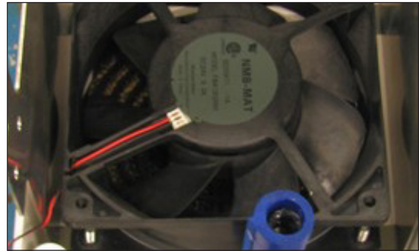
Figure 140 - Step 7 Wire position
