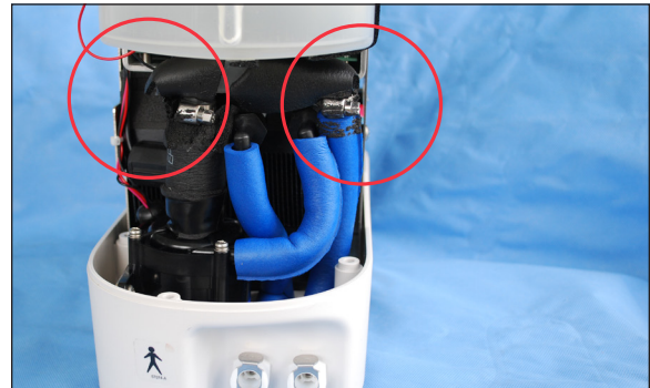
Figure 58 - Step 1 connect tubing to reservoir with clamps
