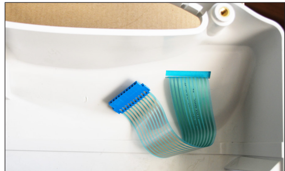
Figure 44 - Step 1 Thread cable through slot
