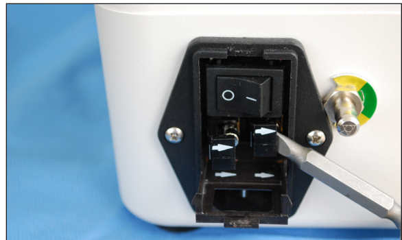
Figure 93 - Step 2 Match arrow direction
