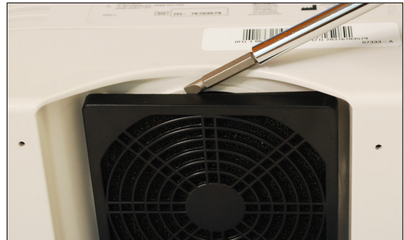
Figure 5 - Step 2 Pry off retainer
