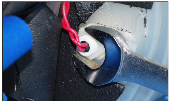
Figure 48 - Step 5 Unscrew float switch mounting nut
