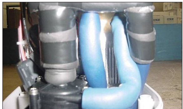
Figure 88 - Step 12 Apply electrical tape around insulation
