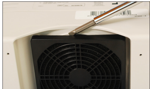
Figure 5 - Step 2 Pry off retainer
