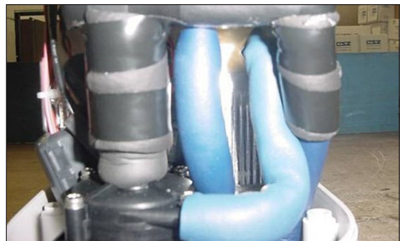
Figure 88 - Step 12 Apply electrical tape around insulation
