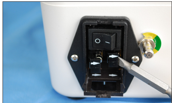
Figure 93 - Step 2 Match arrow direction
