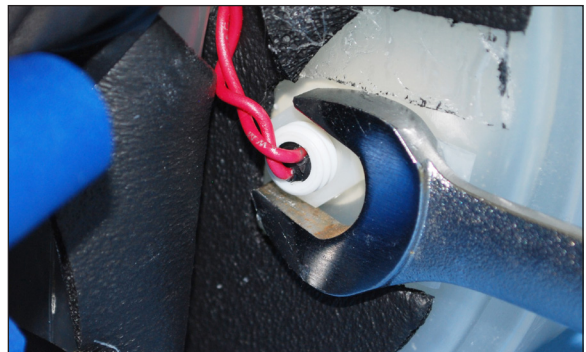
Figure 48 - Step 5 Unscrew float switch mounting nut
