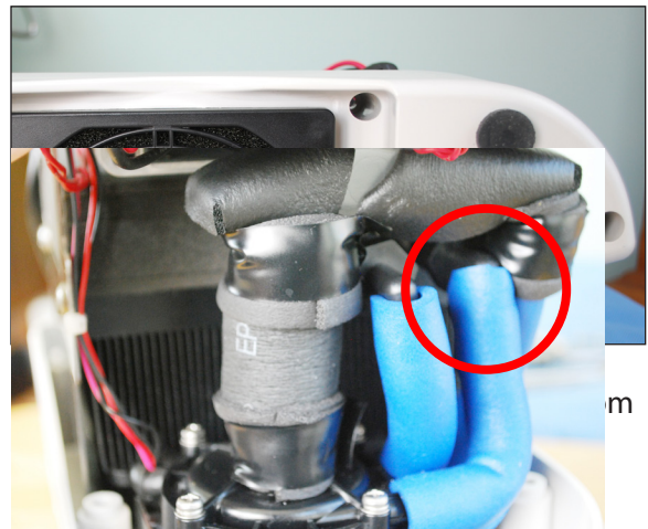
Figure 67 - Step 8 Remove inlet tubing
