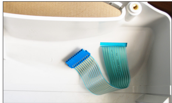
Figure 44 - Step 1 Thread cable through slot
