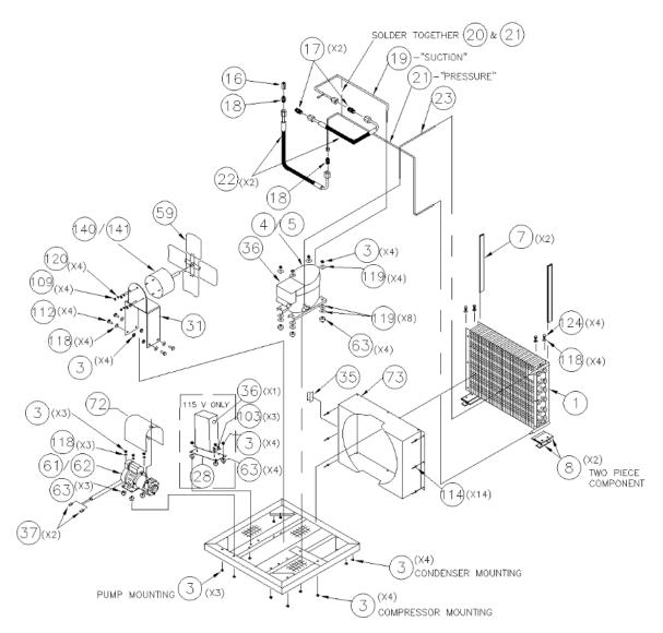
FIGURE 4-3, BASE ASSEMBLIES AND PARTS
