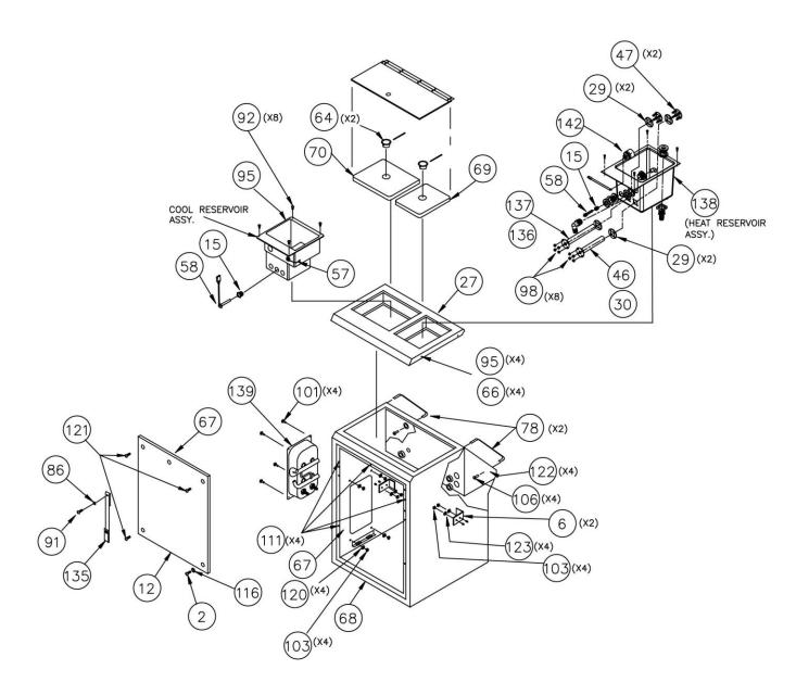
FIGURE 4-2, BACK ASSEMBLIES AND PARTS
