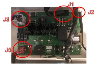
Figure 10 – Top View of Power Board in Place
