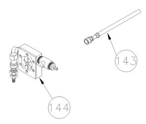
FIGURE 4-4, DRAIN HOSE AND FLOW INDICATOR
