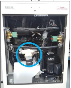
Figure 3-1 Water Filter Assembly
