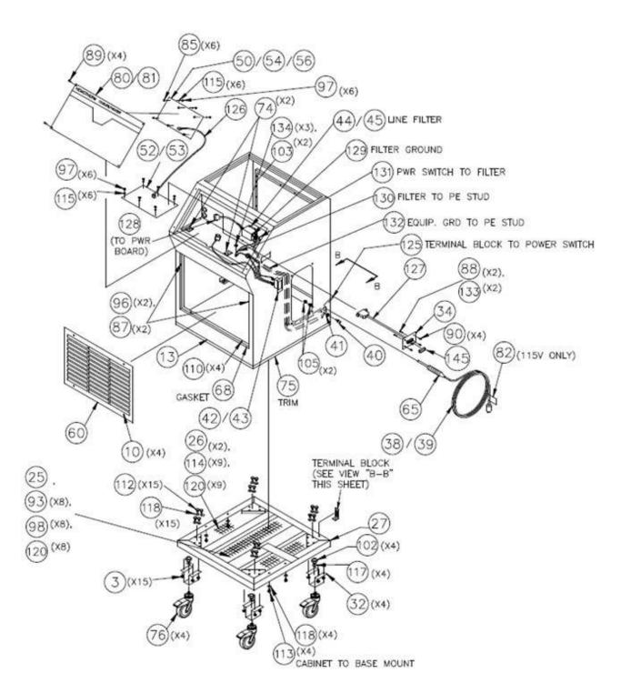
FIGURE 4-1, FRONT ASSEMBLIES AND PARTS
