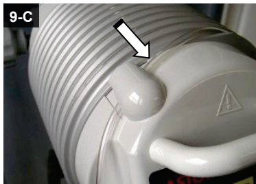
Fig. 9: Inserting of the infusion extension (continuation)
